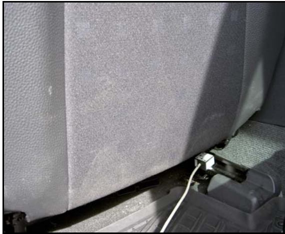
Figure 18. Accelerometer on the seat guide on the floor.
