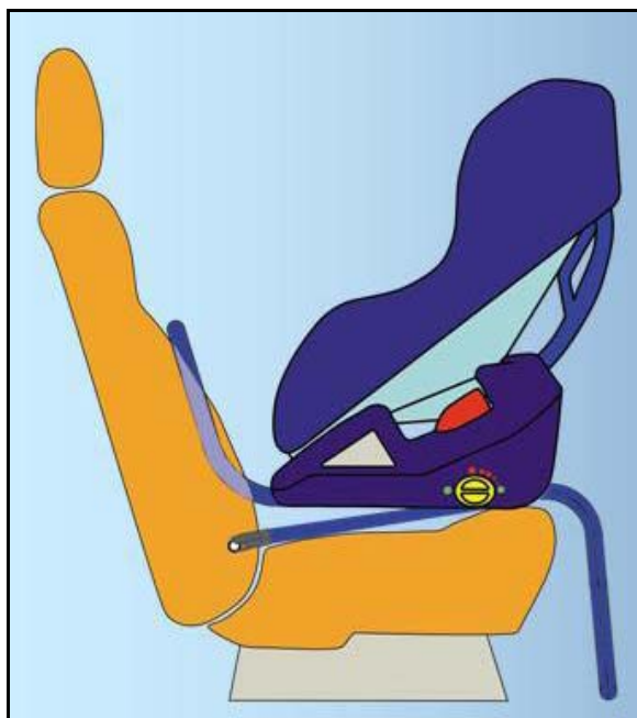
Figure 9. The main attachment is made by connecting the child seat to ISOFIX-bars in the car seat. (Fair Srl)
