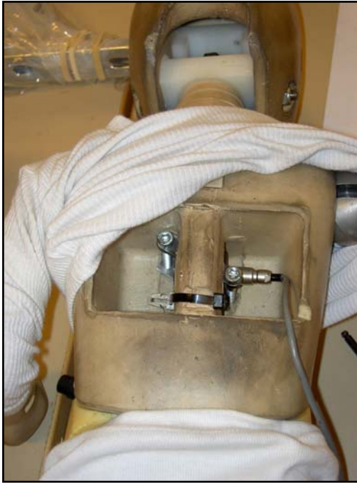
Figure 15. Accelerometer fastened in dummy
