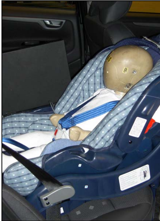
Figure 14. Dummy placed in infant safety seat with base from AKTA Graco
